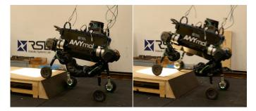
Fig. 1. The quadrupedal robot ANYmal equipped with four non-steerable, torque-controlled wheels, driving up a step 0.2 m high (over 40 % of the legs length) and a  $65^{\circ}$  slope using our TO framework.
