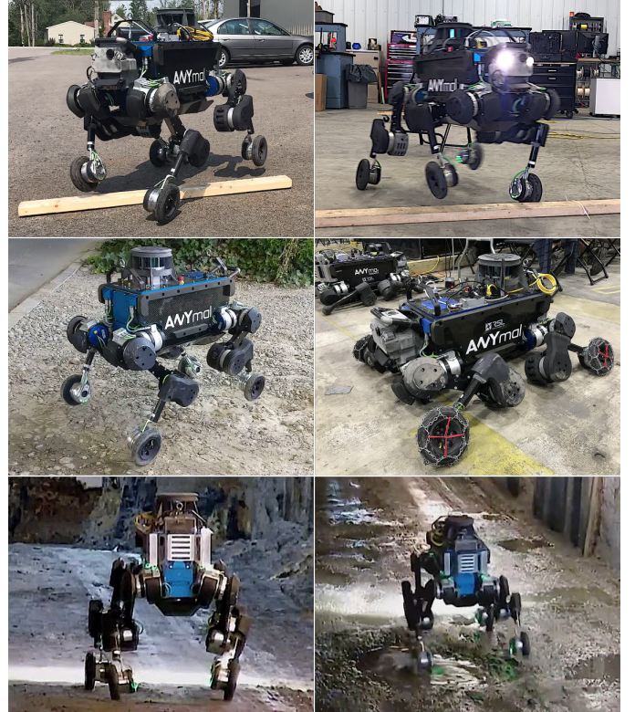
Fig. 1. The fully torque-controlled quadrupedal robot ANYmal [4] equipped with four non-steerable, torque-controlled wheels. The robot is traversing over a wooden plank (top images), on rough terrain (left middle image). In addition, the robot rapidly maps, navigates and searches dynamic underground environments at the DARPA Subterranean Challenge (lower images), and the robot's wheels are equipped with chains to traverse the muddy terrain (right middle image). A video can be found at https://youtu.be/ukY0vyM-yfY .
